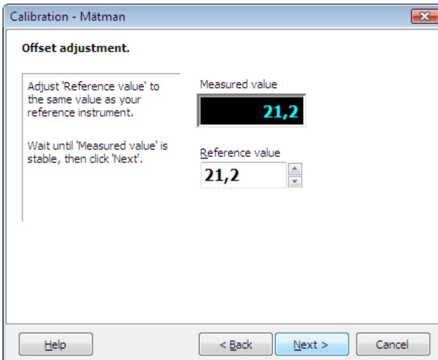
Use this method when you are normally measuring values within a narrow range, and have no possibility to reference measure at two levels.
