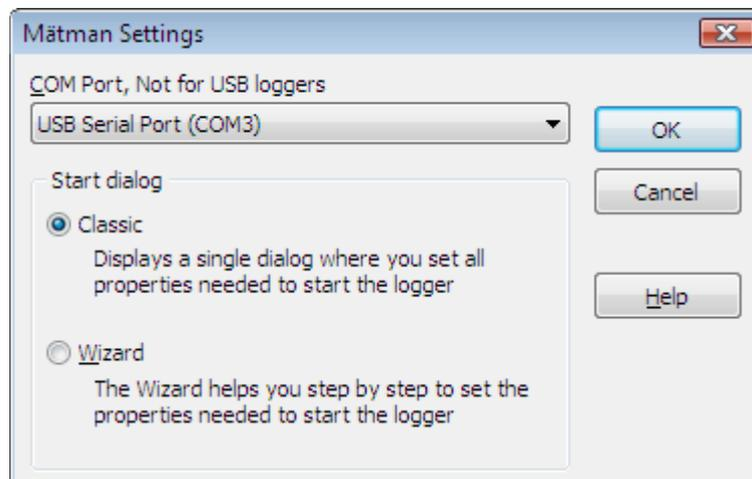
When you have selected a free serial port, check if you can make contact with Mätman. The easiest way to do this is to click the “Show” button, displaying the current measurement value in Mätman.
