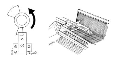
The sensing periods in comparison to weft yarn speed during insertion.
