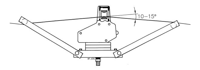
3. A flag is fitted on the main shaft. The light switch should be fitted so that the flag passes through the slot once every pick. The distance between the bottom of the slot of the light switch and the flag must not exeed 4 mm. The flag width must be about 30–45° by 360 picks/min and 45–60° by 500 picks/min. The flag must pass through the slot during the last part of weft insertion.
