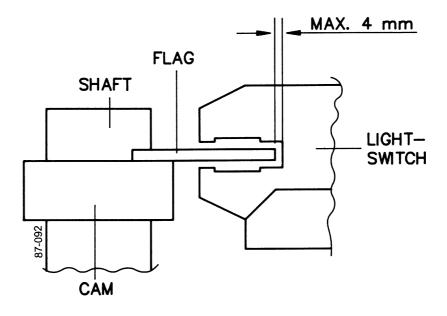
If the ANTI-function is used it is advisable to fit an extra flag which passes through the light switch before the transfer point. The extra flag will make it possible to detect an extra faulty yarn also if it is dropped by the transfer.
