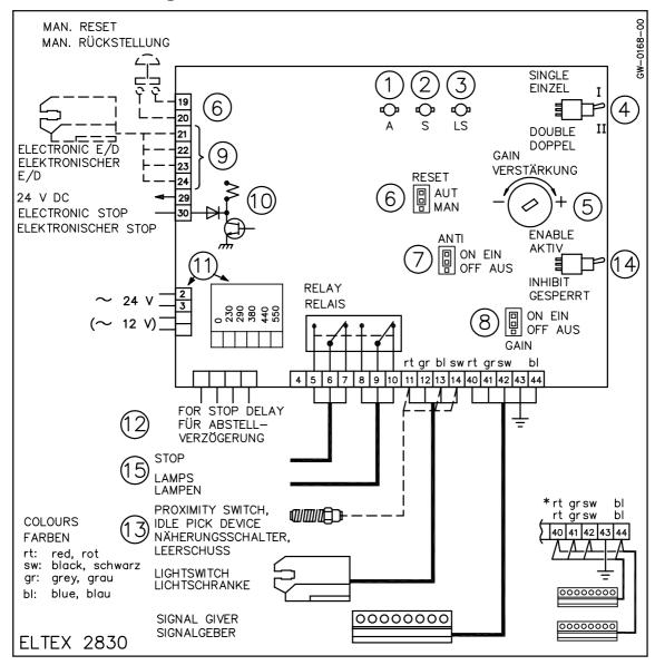
The relay is energised when the machine is running and drops when there is a weft fault.
