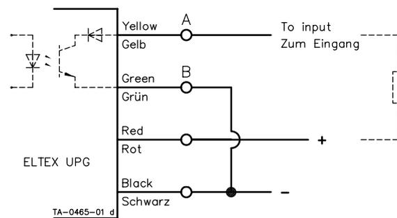
Configured as NPN open collector for input with pull-up resistor; low when yarn is not moving.
