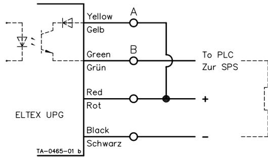
Configured as PNP output for PLC; high when yarn is not moving.
