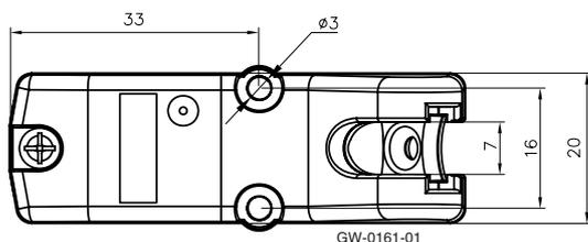
The UPG yarn break detector is fitted on the machine with two screws, maximum diameter 3 mm.
