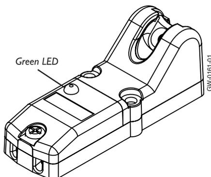
The UPG is a small, general-purpose thread break detector in a robust metal housing. It works on the piezoelectric principle, detecting the yarn movement.
