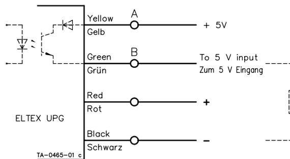
Configured as opto-coupler output; high when yarn is not moving.
