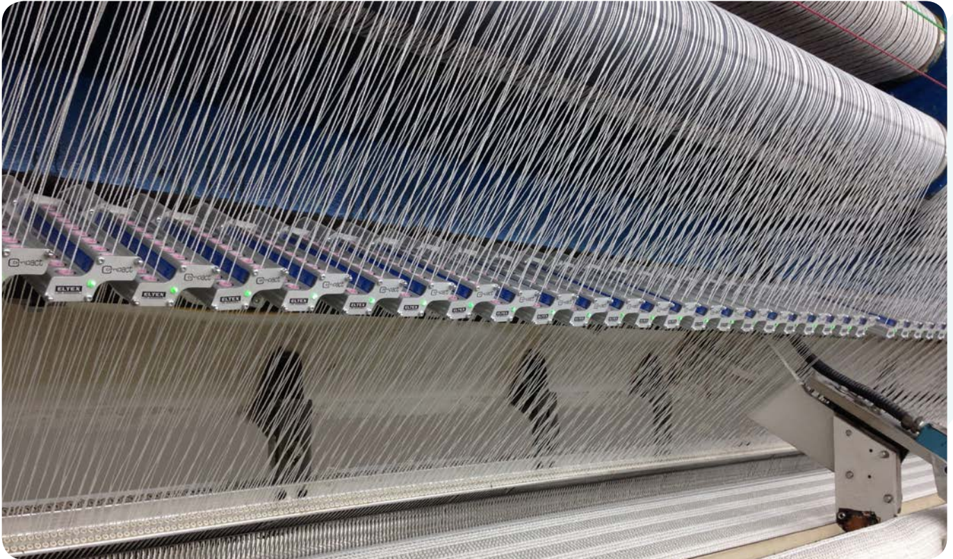
Compact sensors installed on a tufting machine.
