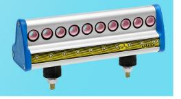
G3s is a yarn break sensor that uses piezoelectric technology to detect yarn movement (not presence) of all types of yarn in many different applications.
