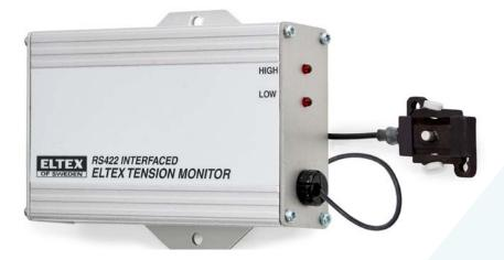
The Eltex Electronic Tension Monitor (ETM) is an on-line device for sewing machines and similar applications. The device monitors the thread tension and also acts as a thread break detector. It enables the operator to keep the thread tension within the desired tension range for best operation and quality of the seam. The ETM422 communicates through an RS422 interface to a host computer. This allows the user to set limits and to watch alarms and readings on the computer display.
