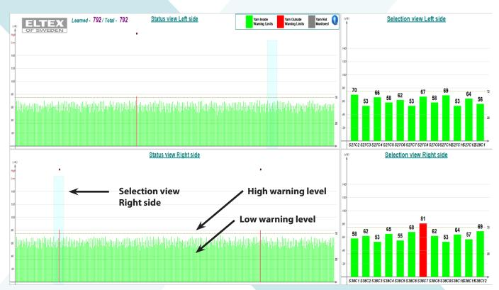
The yarn tension values from all yarns are continuously updated and displayed on a large screen. Tension values outside the warning level will be indicated both on the sensor's LEDs and on the screen. It is possible to expand a selection of the display to have a detailed view including the position ID and the cN value for the yarns in this sector.
