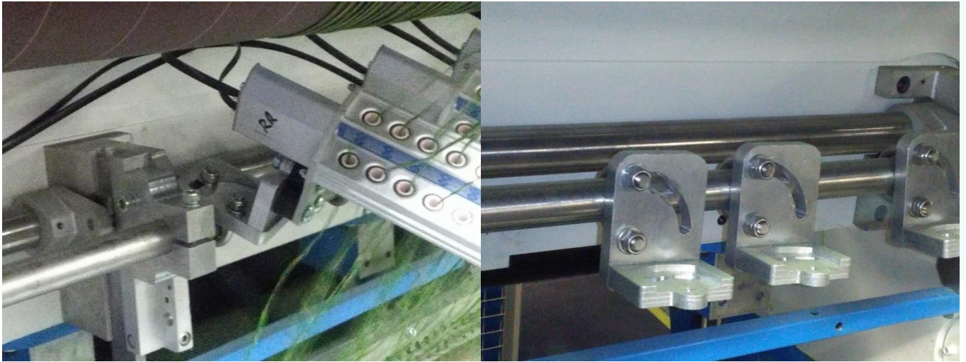
Advanced construction with both vertically and horizontally adjustable brackets.
