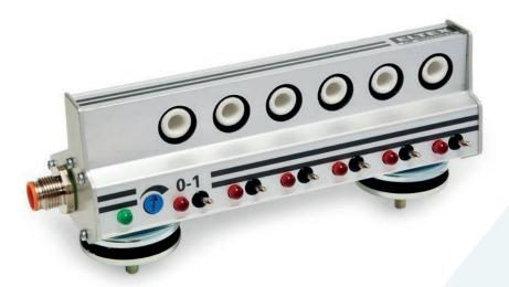
This thread sensor is designed to monitor up to 6 intermittent running threads on automatic sewing machines. The eyelets are scanned electronically. It detects both broken and continuously moving threads.
