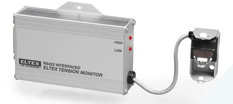
The Eltex Electronic Tension Monitor (ETM) is an on-line device for sewing machines and similar applications. The device monitors the thread tension and acts as a thread break detector. It enables the operator to keep the thread tension within the desired tension range for best operation and quality of the seam. The ETM422 communicates through an RS422 interface to a host computer. This allows the user to set limits and to watch alarms and readings on the computer display.
