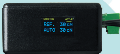
Central unit with buttons for settings and a display to show set tension value and actual yarn tension value.
